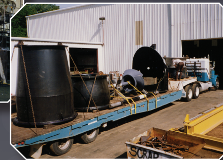
Circulating Water Pump -Sandblasted, replaced bushings and bearings, machined flanges to reclaim fits. Applied coating, precision aligned and dowelled flanges, dis-assembled and delivered to customer.
