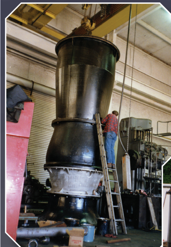
Circulating Water Pump -Sandblasted, replaced bushings and bearings, machined flanges to reclaim fits. Applied coating, precision aligned and dowelled flanges, dis-assembled and delivered to customer.
