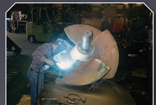
Pump Impeller Repaired with bronze build up
