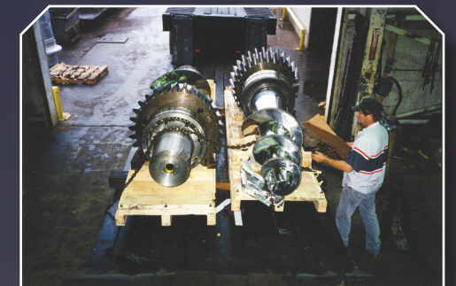
Rubber Extrusion Screws -Inspected, repaired, and replaced bearings and seals
