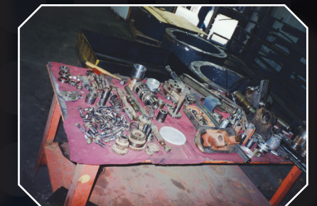
Cincinnati Vertical Mill- Removed knee, disassembled, replaced bearings, seals and repaired as needed
